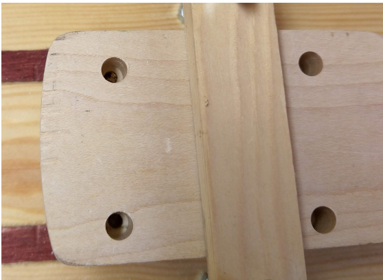
4mm & 6mm stepped holes ready for inserts
