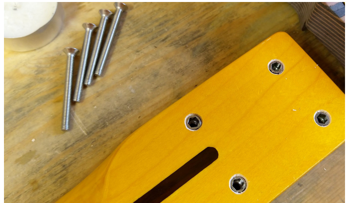
Inserts in place ready to re-fit the neck
